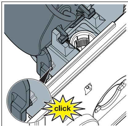
► Let the control engage in the mechanism.
