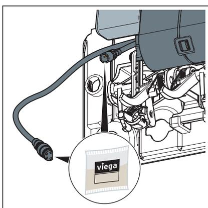
► Apply the silicon grease to all connections of the control.
