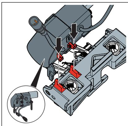
► Place the control on the mechanism.
