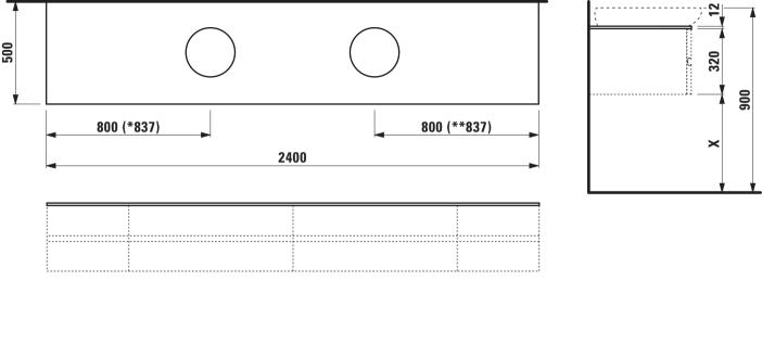
\* = Only II Bagno Alessi One \$1897.3 with shelf at left side / \*\* = Only II Bagno Alessi One \$1897.3 with shelf at right side X = The exact hight must be set during installation.
