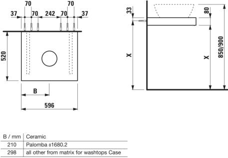
X =The exact height must be set during installation.
