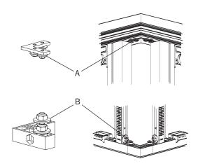
• Push the corner joints of the side parts (A, top and B, bottom) into the longitudinal parts and tighten the screws.
