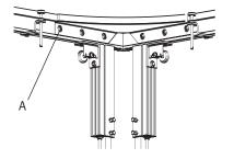
In the case of oval or octagonal bathtubs, fillers have to be installed in addition.
