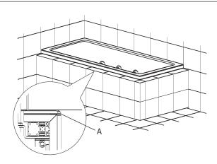
Tip: When mounting the tiles, it is recommended to use a plastic or metal profile bar (A).
