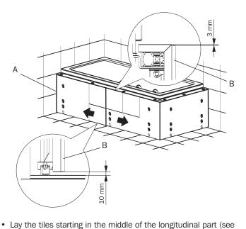
Note I: The tiles (B) shall be mounted with a gap of at least 3 mm (A, see detail) around the front panels. That gap guarantees the free movement of the front panels and shall be flexibly sealed later on.
