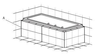
Point the gaps (A) between the front panels and the continuous edge below the bathtub rim with sealing material and let them rest until the sealing material has hardened completely (see manufacturer's instructions).
