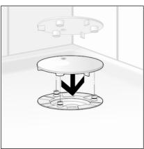
Press the cover plate onto the three fixing points.
