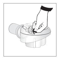
Insert closing plug flush with the surface.
