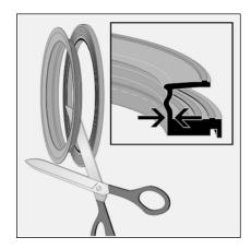
Cut the seal into two pieces at the sealing bead.
