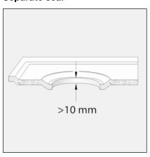
If the shower tray floor is thicker than 10 mm, you must separate the seal as follows:
