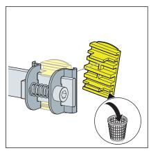
Remove the plug-in pieces of the parallel connector and discard.
