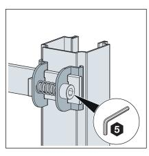
■ Use the Allen key (SW 5) to mount the parallel connector on the closed side.
