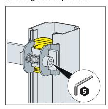
Mount the parallel connector with the plug-in piece on the open side of the mounting rail. Use an Allen key (SW 5).
