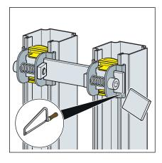
For installation depths smaller than 145 mm, use a hacksaw to cut the tab of the parallel connector to length.
