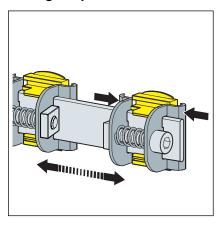
Gently compress the tendon and move it to adjust the distance of the tendons of the parallel connector.
