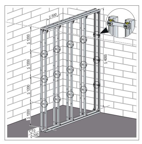
Steptec partition wall (max. height 4 m). Installation depth (max. 145 mm). Distance between parallel connectors max. 1.2 m.
