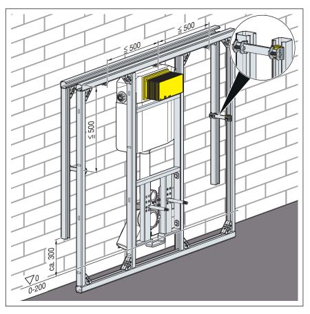
Mounting the Steptec WC module with a max. installation depth of 145 mm.
