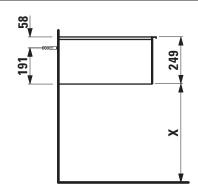
X =The exact hight must be set during installation.
