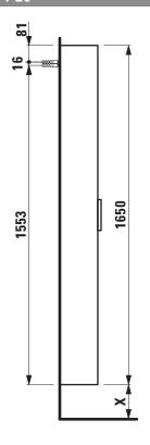
X =The exact hight must be set during installation.
