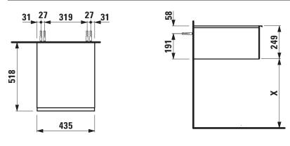
X = The exact hight must be set during installation.
