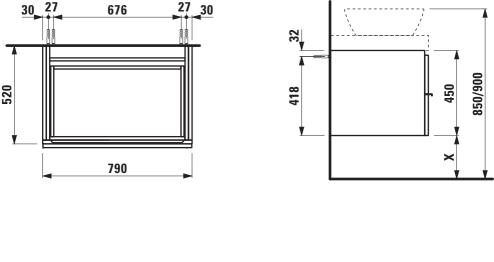
X =The exact height must be set during installation.
