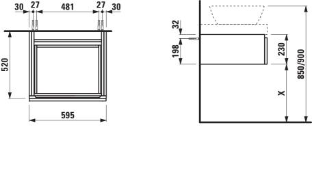
X =The exact height must be set during installation.
